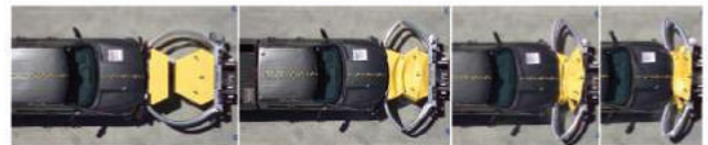
Scorpion II ® Metro TL-2 TMA Impacted by 5,000 lbs (2,268 kg) Pick-Up Truck
