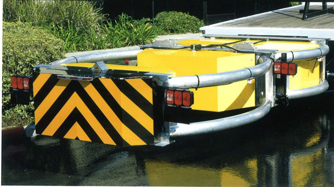
The Scorpion TMA is hydraulically powered and measures 13 feet long when fully extended, making it ideal for stationary and mobile construction zones.
